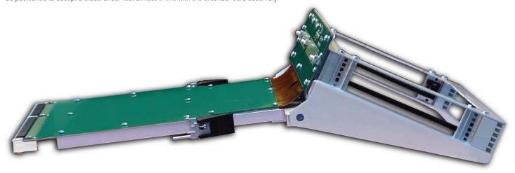
The VPX extender boards are designed to bring a circuit card completely out of a card cage or enclosure so that it can be tested or debugged. This provides access to both sides of the test board. Both the backplane interface and the D.U.T. interface of the extender card provide an alignment key as defined within ANSI-VITA 41.0.
